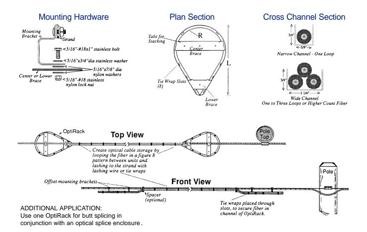
The Moore OptiRack will accommodate a full range of optical cable fiber counts and bend radii. Call a Moore representative for additional assistance in determining channel and radius requirements.
